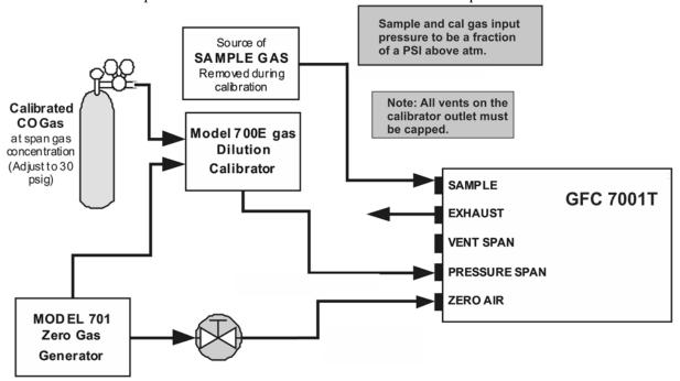
Figure 9-3: Pneumatic Connections – Option 50A: Ambient Zero/Ambient Span Calibration Valves
